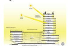
The narrow footprints of the north tower and south bar allow for ample daylighting; where the two masses engage the central atrium space, daylighting is borrowed from the atrium using interior glazed walls. - Photo Credit:
