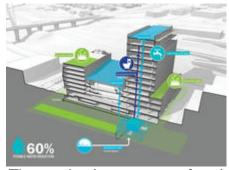
The north wing upper roof and atrium rooftop serve as water collectors for the rainwater reuse system, while the south wing and lower roof on the north wing provide habitat for native species. - Photo Credit: SERA Architects
