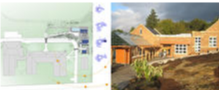
Climate analysis (left) influenced the building orientation which shelters the entry (right) from prevailing winds - Photo Credit: Opsis Architecture
